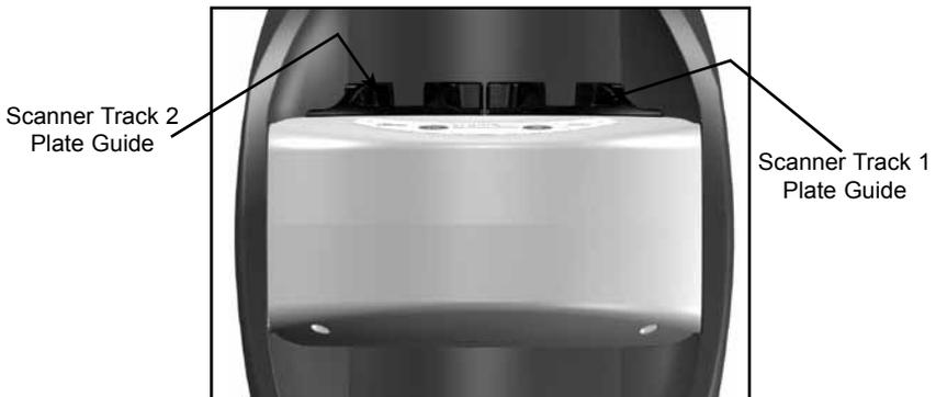
Figure 8. ScanX with a full Complement of Plate Guides in Place.
